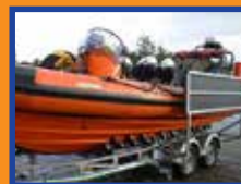
Fully equipped 6.8m RIB with twin 90hp engines and qualified voluntary crew.
